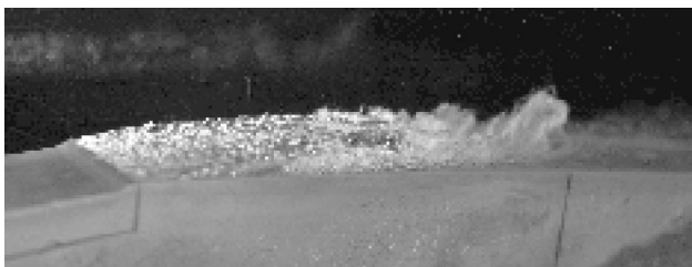
Fig. 8 Photograph of sheet cavitation
