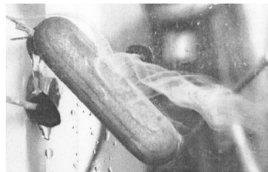
Fig. 3 Vortex visualization by dye injection, for Re=1000 , behind a generator of the first column
